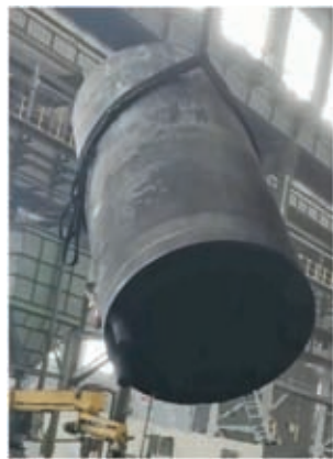
图8 百吨级球墨铸铁核乏燃料容器铸件 Fig. 8 100-ton grade ductile iron casting container of the spent nuclear fuel
