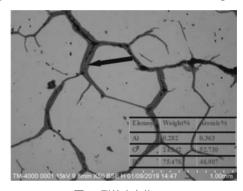
图4 裂纹夹杂物EDS Fig. 4 EDS of crack inclusion
