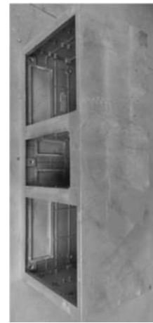
图11 优化方案的铸件图 Fig. 11 Produced casting using improved casting process
