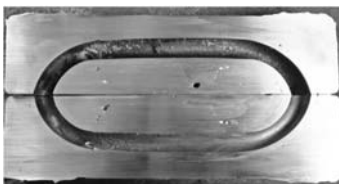
图12 剖开后的铸件 Fig. 12 The casting after being split
