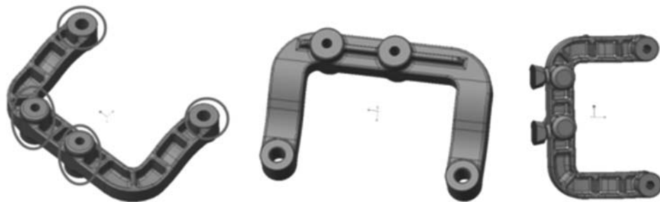
图7 A产品的冷铁工艺方案 Fig. 7 Chill process of new product case A
