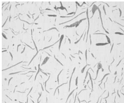
图3 使用低硫低氮增碳剂的试样石墨形态 100× Fig. 3 Graphite morphology of samples using low sulfur nitrogen recarburizer
