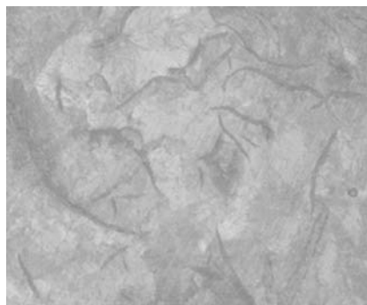
图6 使用高硫高氮增碳剂的试样基体组织 500× Fig. 6 The metallurgical structure of the sample using high sulfur nitrogen recarburizer
