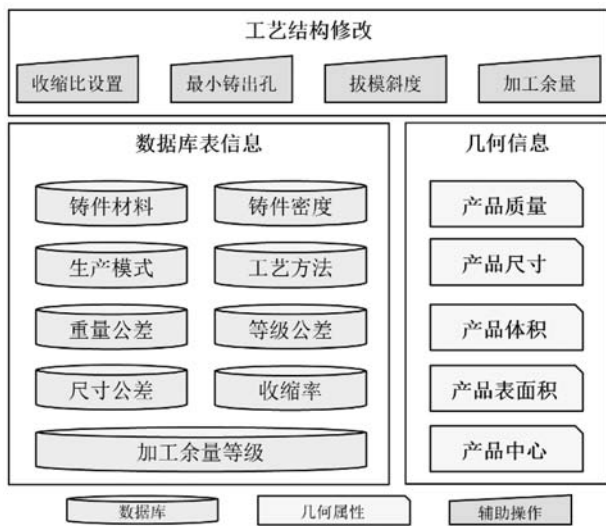
图4 产品零件可铸造工艺分析前置处理属性和操作 Fig. 4 Product part castable analysis preprocessing properties and operations
