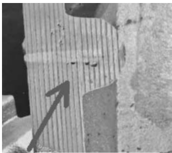
图4 铸件缩孔 Fig. 4 Shrinkage of the casting
